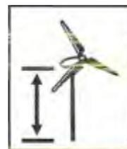
**Wind generator.** The blades and associated mechanical and electrical conversion components mounted on top of the tower whose purpose is to convert kinetic energy of the wind into rotational energy used to generate electricity.
