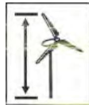
**Tower height.** The height above grade of the fixed portion of the tower, excluding the wind generator.
